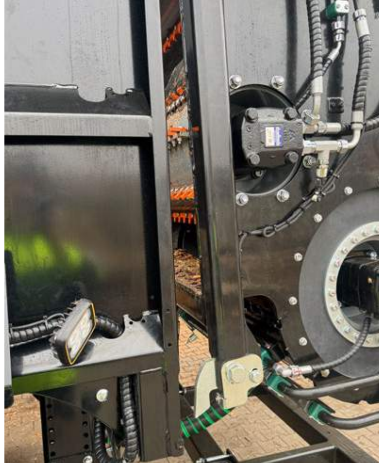
Rear flap can be opened for maintenance
